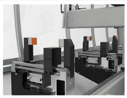
On request are available pneumatic vices with independent movement/positioning. On request, the working area can be equipped with the "pendular machining" function to allow the operator to load/unload profiles in masked time. The option requires the installation of a second pneumatic retractable stop on the right of the working area. The motorized chip conveyor is installed in the base.
